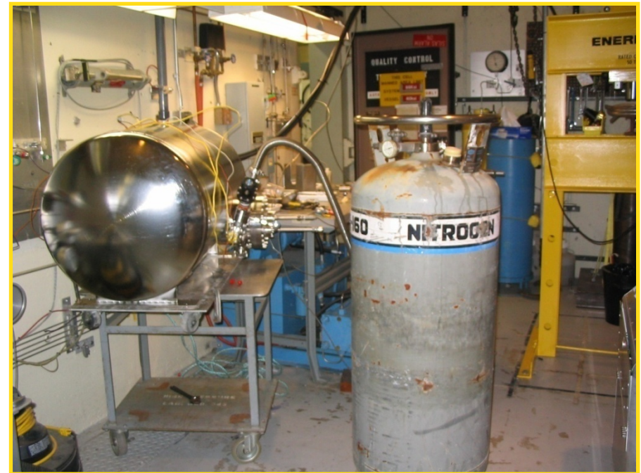
Cryogenic dormancy test setup
